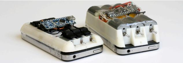
**Figure 2:** Our pocketOuija, here two versions of it, actuate the user's finger by moving a clear foil on top of the device's touchscreen (here an iPhone).
