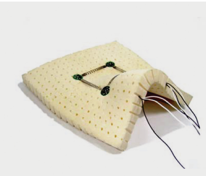
Figure 1. Shape memory alloys, which have been used to alter the shape of airfoils [4], have also been employed to create interactive surfaces that can be reprogrammed for real-time computer modeling of objects and spaces, and the construction of adaptable interfaces [5].
